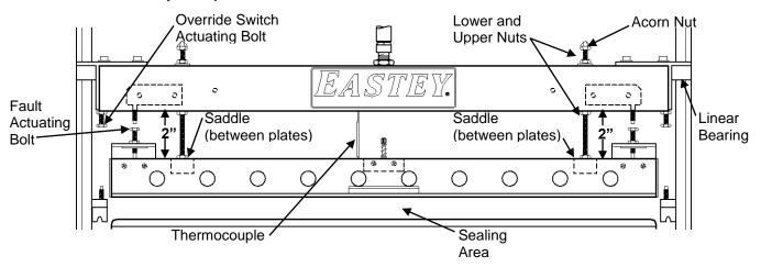
5. If the film pressure is unequal, loosen the upper and lower nuts holding the seal bar saddle in place only in areas where pressure is unequal.
