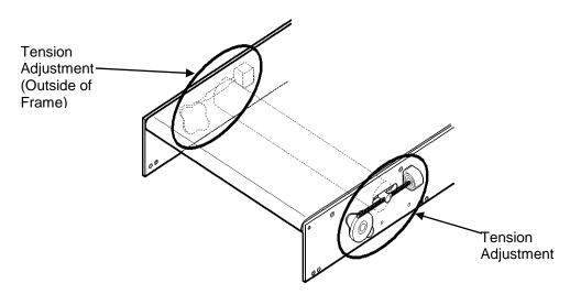
Ideally the conveyor shaft should be adjusted so that when correct tension is achieved, the shaft is near the center of adjustment slot. Before beginning adjustment, measure these distances to place the conveyor shaft near the center of adjustment.
