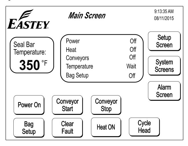
Once the electrician has stated that all electrical work is complete and the air line is connected to the regulator and providing 60 PSI and 3.5 CFM, make sure all shipping ties are removed and all personnel are clear of the equipment, then power up the sealer and run it through a cycle by performing the following.
