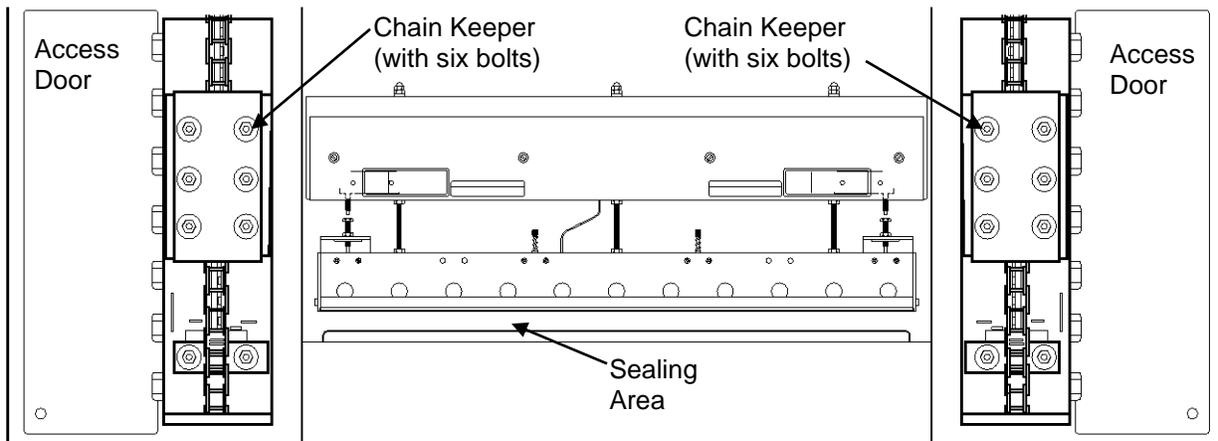
4. Temporarily remove the chain keepers: use a  $\frac{1}{4}$  inch hex wrench to loosen the bolts securing the chain keepers. There are six (6) bolts on each side of each of the chain keepers.
