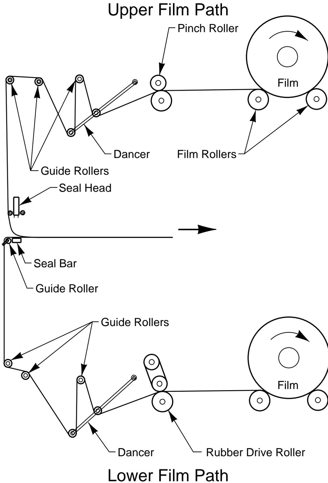
8. Pull the upper film in front of the upper seal bar, then around to the back side of the seal bar.
