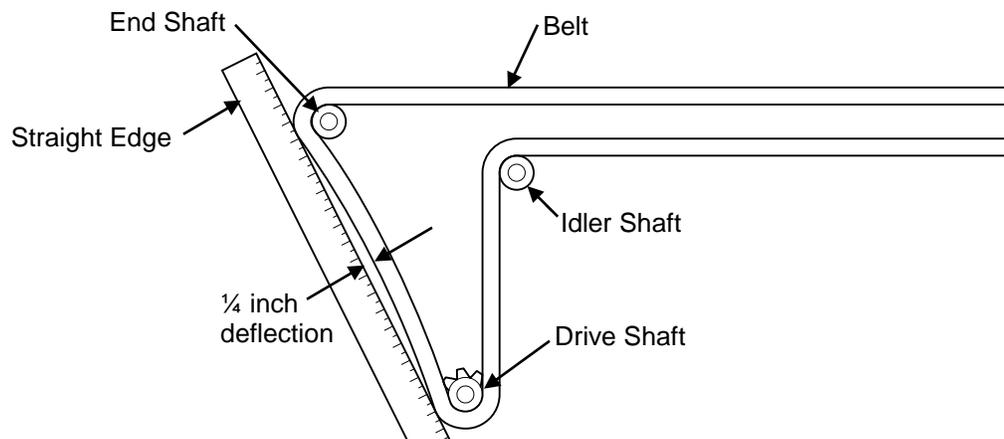
4. When the conveyor tension is correctly adjusted, re-tighten the lock nuts.
