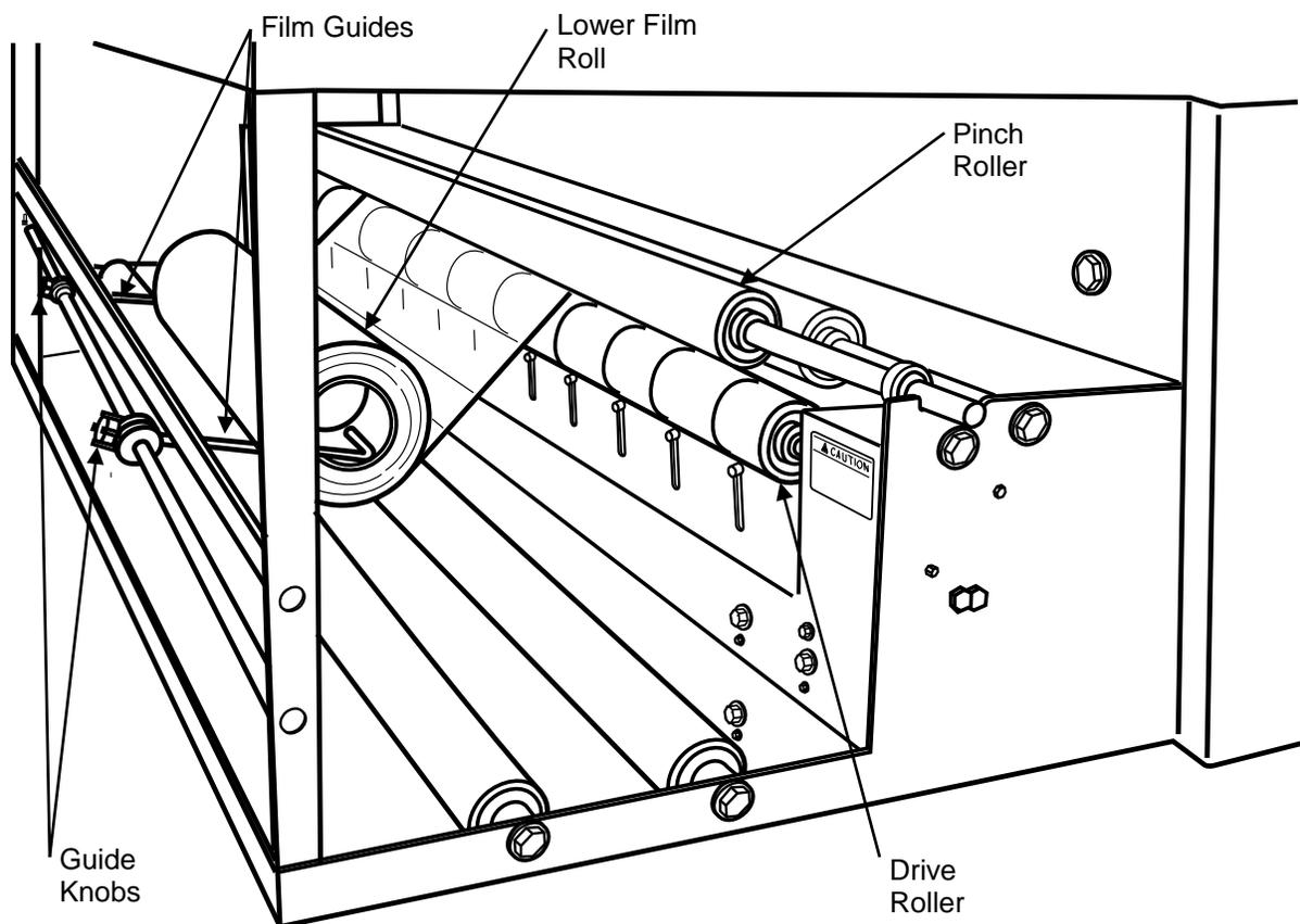
3. Place the film on the support rollers with the film coming off the bottom as shown.
