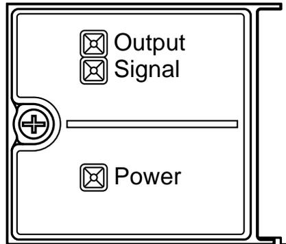
**NOTE:** When properly set up and operational, the red and green lights on top of the eye will be illuminated. Breaking the beam will cause the "Signal" light to go out and the yellow "Output" light to turn on. The Signal light will come back on when the beam is reconnected and the yellow Output light will turn off.
