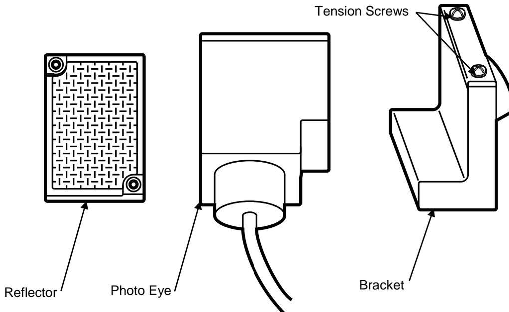
If the beam is not properly lined up on the reflector, the output and signal lights will not be illuminated. To adjust the beam into the reflector, loosen the two tension (Phillips) screws on the top of the mounting bracket (see the illustration above) and move the eye by hand until the red light is centered on the reflector.
