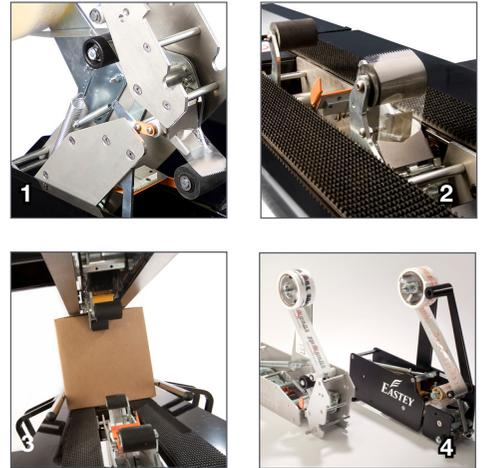
1. Top and bottom tape heads are interchangeable and tip back for easy threading
