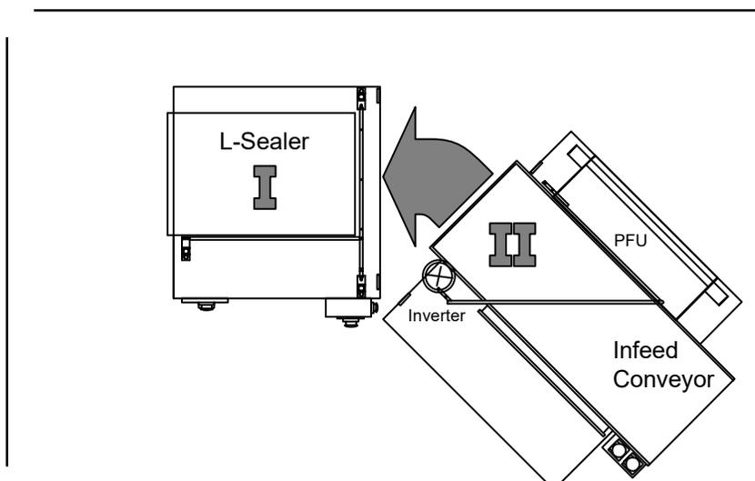
Adjust the leveling legs to support the PFU/Infeed Conveyor/Inverter module and level the Infeed Conveyor so it is level with the exit conveyor, and also level along both the machine-direction axis and transverse direction axis. Carefully align holes in attachment flanges with bolt holes in machine base. Use the bolts provided to fasten the two sections together.
