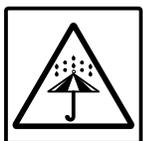
**Moisture hazard.** Keep equipment dry. This equipment is designed for indoor operation in a typical clean, dry factory environment, protected from rain and moisture. Do not operate the machine in any extremely wet or oily environment that may exceed operating specifications.
