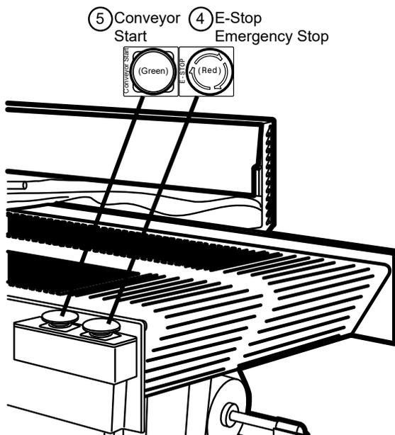
5. **Conveyor Start** — Large, green, palm button to start the conveyor for one-item-at-a-time operation. See instructions for running one product at a time later in this User Guide.
