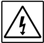
**Electrical hazard.** Indicates electrical danger. Allow only a trained electrician to open the door or cover of the electrical panel or box. Shut off electrical power before attempting to open or work in the electrical box, junction boxes, or other electrical components of the unit.
