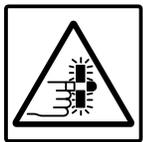
**Cut or shear hazard.** Do not place your hands or any object on the sealing or cutting zone at any time. Shut down the machine before performing maintenance, parts replacement, or troubleshooting in these zones.
