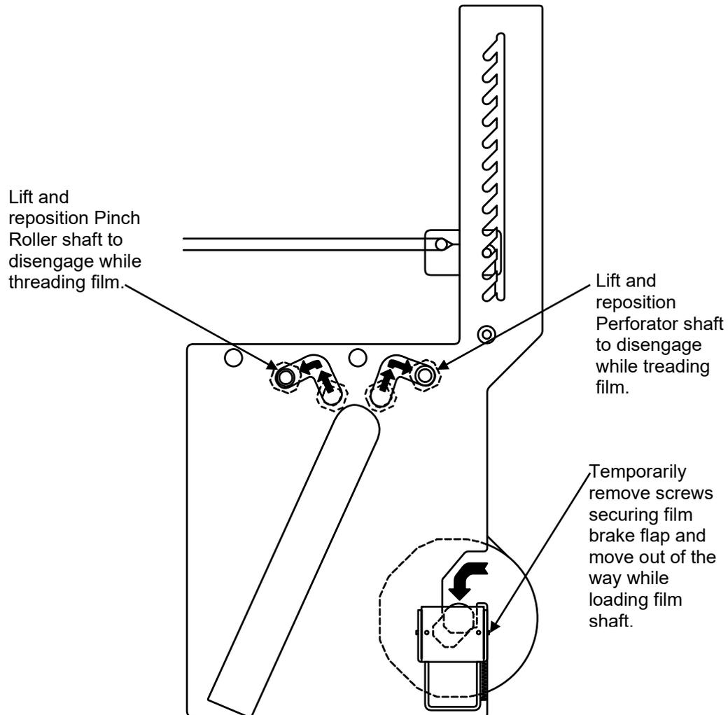
3. Place the film roll on the film roller shaft at the bottom of the film unwinder (shown in the illustration above). Place the center-fold toward the infeed end of the machine. Note that whether the film is A- or B-wind will determine whether the film should roll off from the top or the bottom of the roll. Position the film roll centered on the shaft and tighten the bolts in the film shaft collars to hold the film roll centered.
