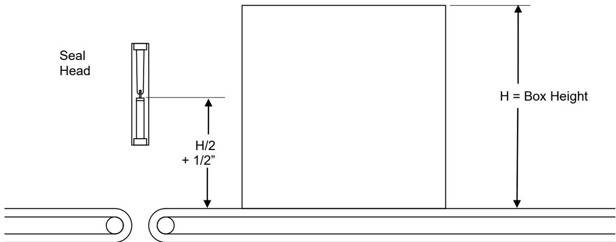
6. While adjusting the seal head height, also change the scrap chain and pinch roller height accordingly. Use the scrap chain height adjustment handle near the center of the Machine Direction seal / cutter to adjust the scrap up or down as needed.
