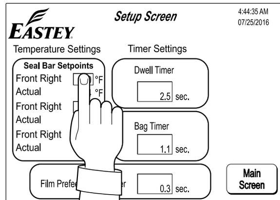
5. The on-screen screen numeric keypad appears. Use the numeric keypad to type the number representing the L-Seal temperature setting or number of seconds for timer, and then touch the Enter button to save your setting and close the numeric keypad window.
