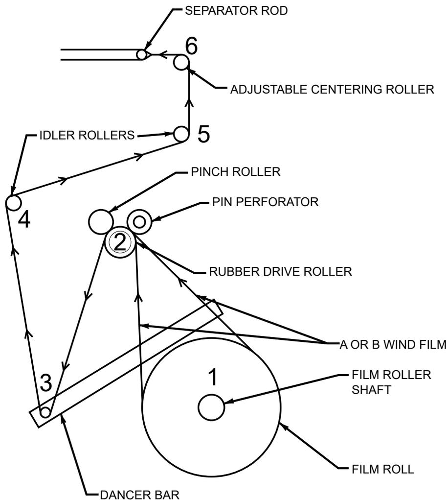
5. Separate the top film from the bottom film with the separator rod and so that bottom film will go below the infeed conveyor and the top will go above.
