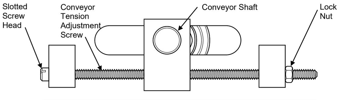
2. Use a flat blade screwdriver to adjust tension.
