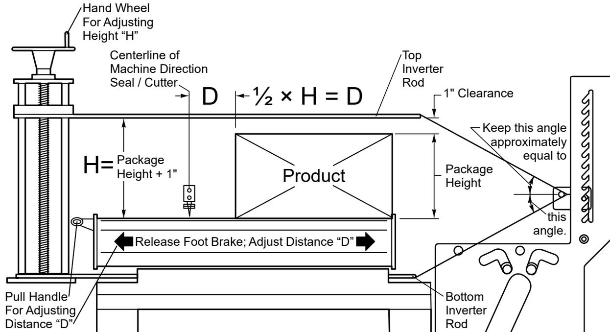
9. To adjust the infeed conveyor position for the width of the product package, release the locking foot near the center of the conveyor and the conveyor can be moved freely front to back. Re-engage the locking foot when the conveyor is positioned correctly.
