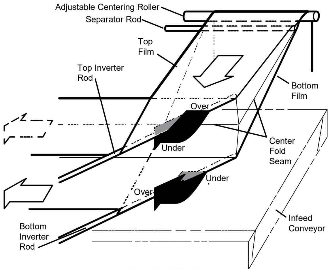
11. Adjust the height of the adjustable centering roller and separator rod if necessary to the center of the vertical distance between the two inverter rods. (See the figure near the top of the previous page.)
