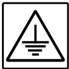
**Ground** symbol. Indicates ground. Use Class-3 (lower than 1000) cable to ground to earth. Incomplete grounding may lead to electrical shock.
