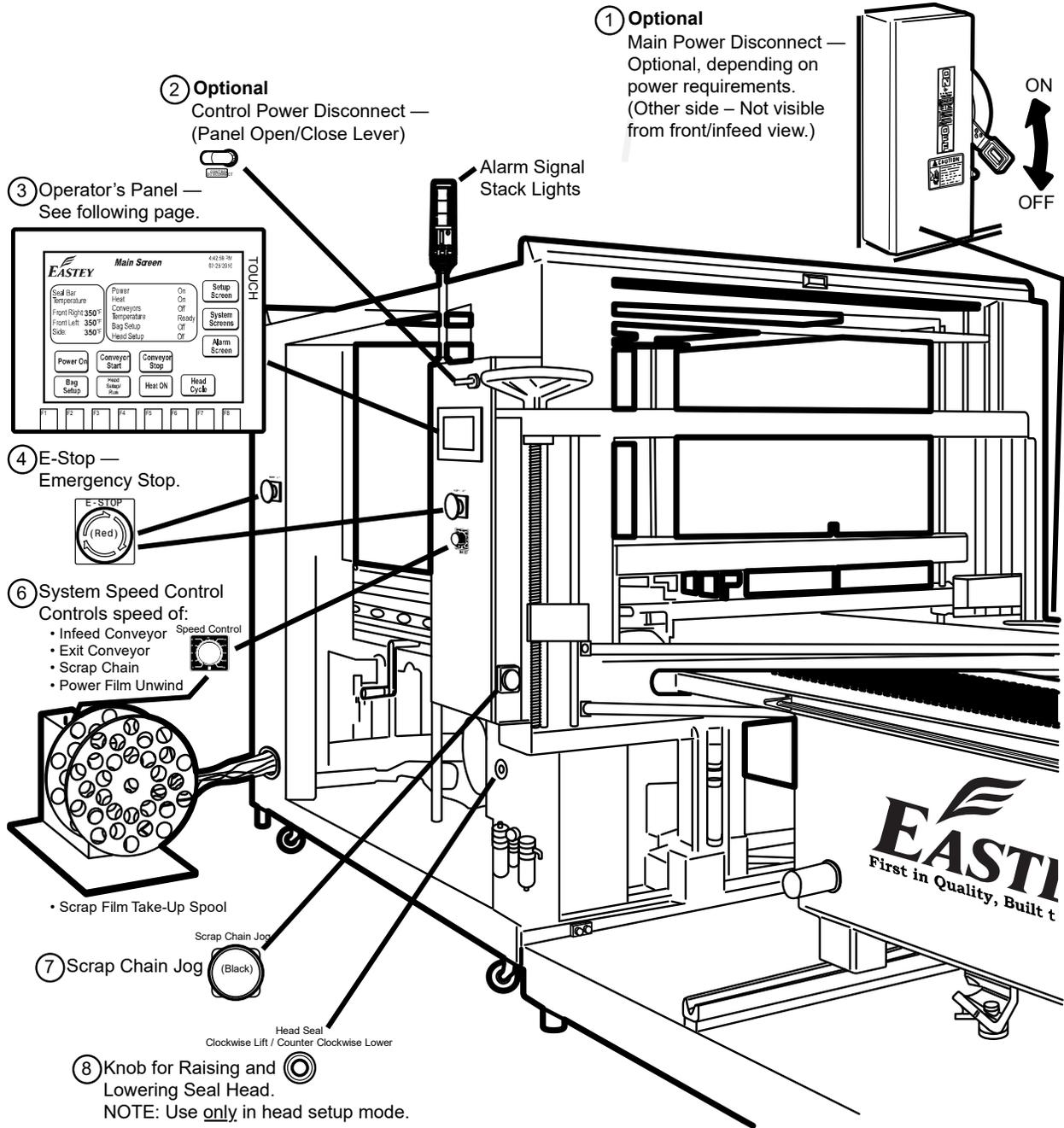
1. **Optional Main Power Disconnect** — For systems with optional 480V power requirements only, a main power disconnect is located on the main electrical box where power enters the system. This switch is a lever with an orange handle.
