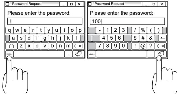
3. When you have entered the password successfully, touch the Setup Screen button and the Setup Screen appears.
