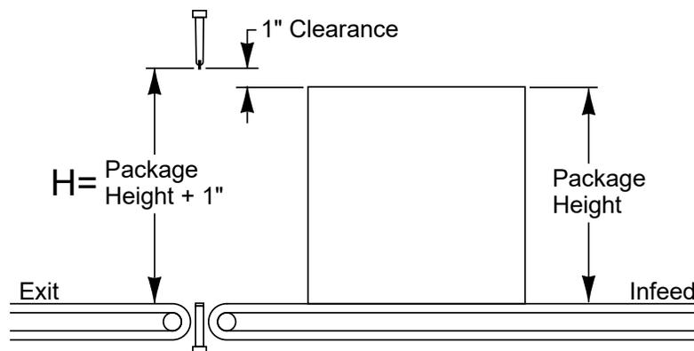
Similarly, allow approximately the same distance, H, between packages, so that the seals occur a distance  $D = \frac{1}{2} \times H$  before and after each package.
