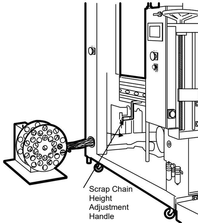
**NOTE:** When adjusting the height of the seal / cutters, it is important to also adjust the height of the scrap chain. Otherwise the seal / cutter could collide with the scrap chain, resulting in damage to the machine.
