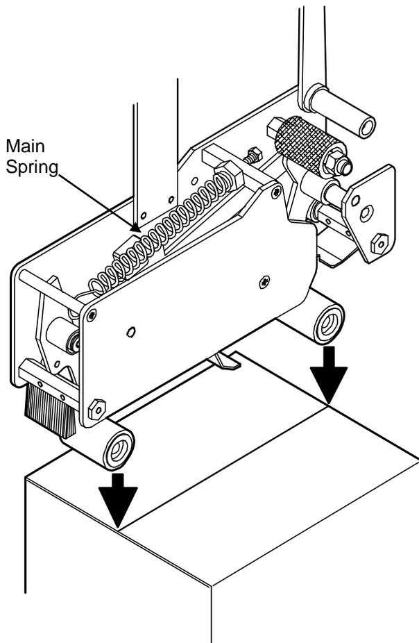
For sealing light weight boxes, decrease the main spring tension. For heavier boxes, increase the main spring tension.
